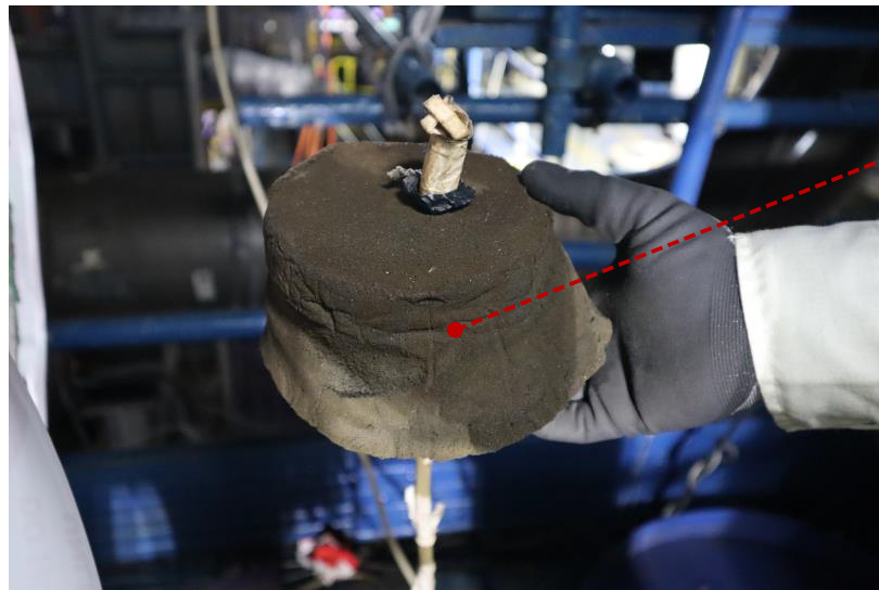
Figure 4: The foam damper used at the bottom end of the 10 cm pipe.
